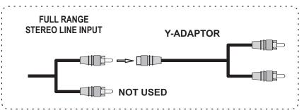
Note: You can use the Radio/CD designated mono line output or a full range stereo line output. For full range stereo line output, you will need an optional "Y-Adaptor" as shown.
